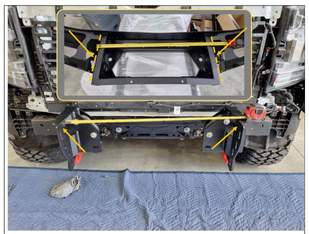
48. Measure the distance between the outside faces of uprights on bar using tape measure. Write distance below for reference if required.
