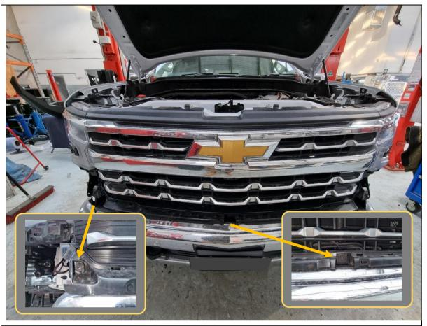
15. Remove 3x 10mm hex bolts along the bottom of the grille. 2x on each end and 1x in the middle.
