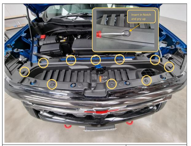
13. Remove 10x plastic push rivets securing the radiator grille cover, by levering centre section upwards using flat bladed screwdriver or trim tool, as shown.
