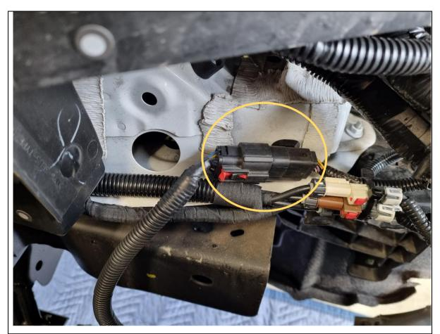
21. On the LH passenger side under the headlight, disconnect the main bumper harness connector.
