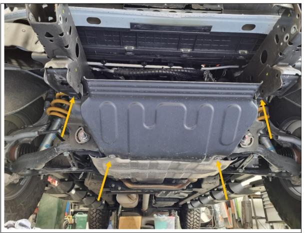
34. Remove the 4x 13mm hex bolts securing the underpanel to the chassis. Retain bolts for re-use.
