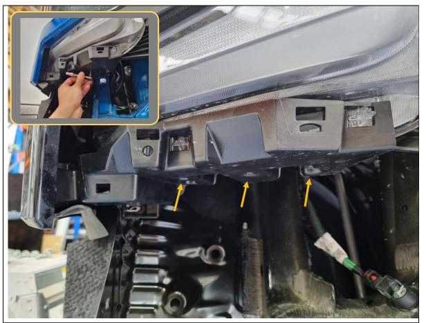
65. Remove the bumper clip underneath the headlight by loosening 3x T15 Torx screws. Do not discard the fasteners.
