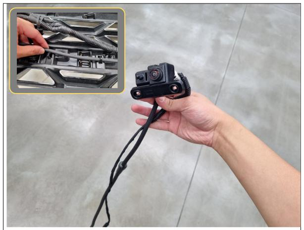
54. Unclip the camera harness and rubber washer hose from the grille.
